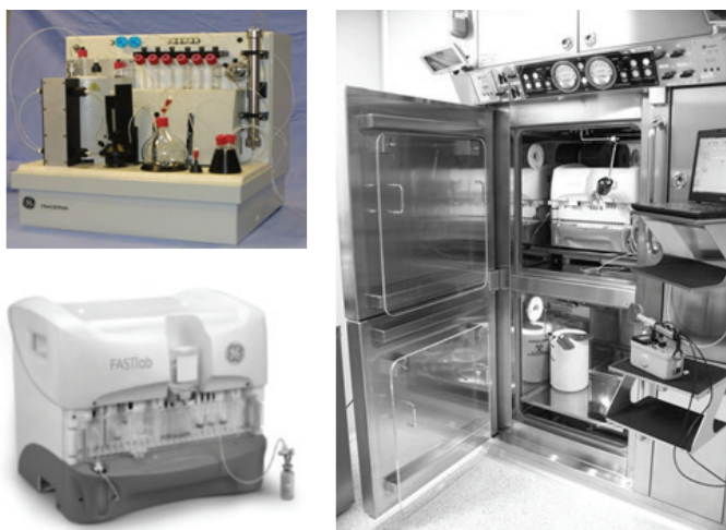
FIGURE 1: FASTlab™ FDG synthesis module (GE Healthcare) (upper left). TRACERlab™ FX C Pro synthesis module (GE Healthcare) (lower left). COMECER BBS-2V Hot-cell with the FASTlab™ FDG module (right).
